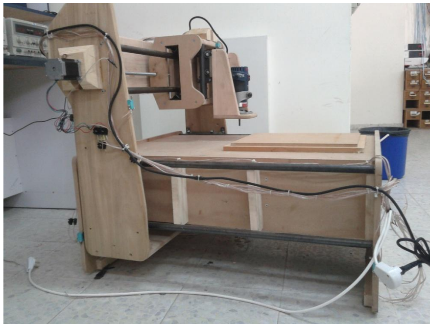
Figure 3- 4 Side view showing X axis of the machine.
